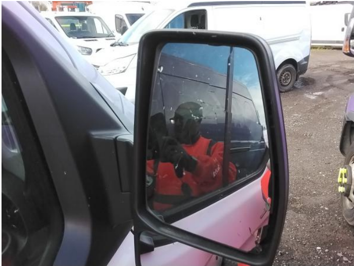
4: Door Mirror Glass os Broken Replace
