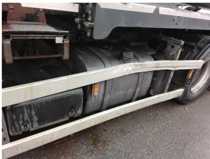
2: Qtr Panel Trim ns Broken Replace
