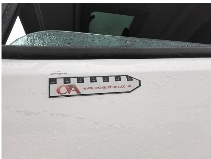
1: Door nsf Scratched Over 25mm Thru Paint
